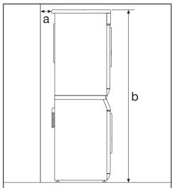
The Miele washing machine can be installed as part of a washer-dryer stack in combination with a Miele tumble dryer. An appropriate "stacking kit\*" is required.
